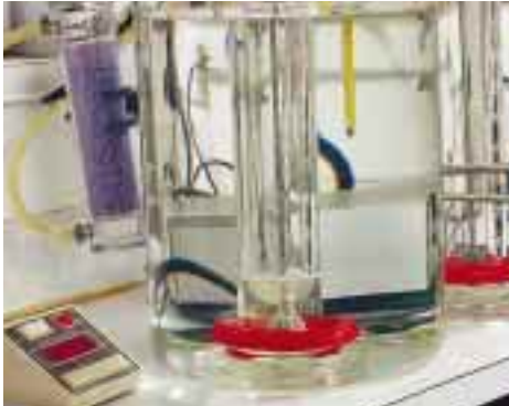
AMSOIL synthetic compressor oils form virtually no foam during ASTM D892 testing.
